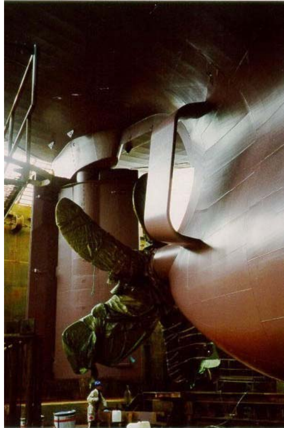
Simplified compensating Nozzle
