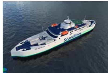
operating conditions, cruising at a speed of 10 knots with zero-emission, and cruising in diesel-hybrid mode at a speed of 16 knots with the support of its generators. The ship will be built according to the class rules of the Lloyd's Register and will have the title of one of the largest battery-capacity ships of around 10 MWh.
